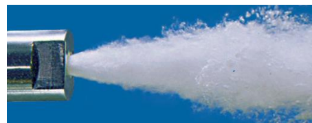
Figure 11 Gas discharge of injection sparger
